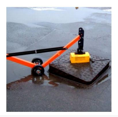
The Manhole Buddy magnetic manhole lifter is designed to lift almost every type of cover up to a maximum weight
